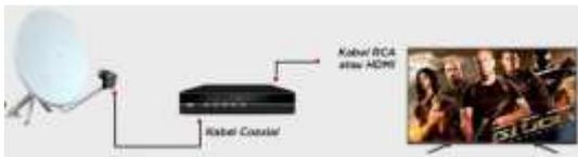
Gambar 19. Diagram Instalasi Receiver dan TV
