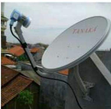
Gambar 8. Dish Antena TV Parabola diameter 45-60 cm
