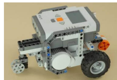
Gambar 7. Pemasangan NXT Intelligence Brick
