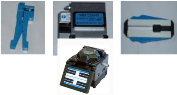
Gambar 5. *Tube Cutter, Fiber Cleaver, Fiber Stripper, Fusion Splicer* (Dari Kiri ke Kanan)
